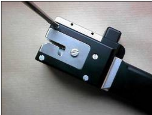
Figure 19. The simple splicer side-cheek – removal
