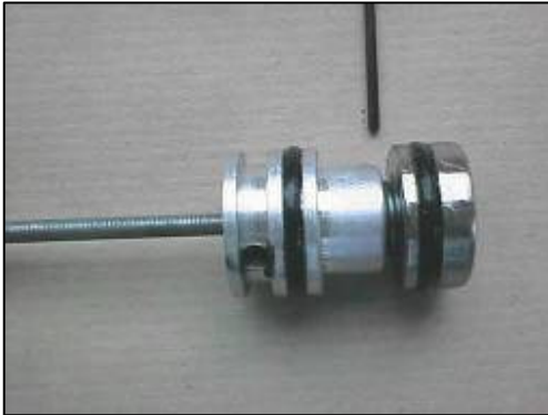
Figure 18. Plug and chamber pad assembly
