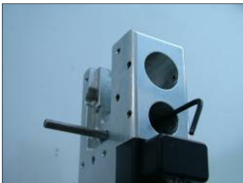
Figure 32. Unlock knife drive shaft
