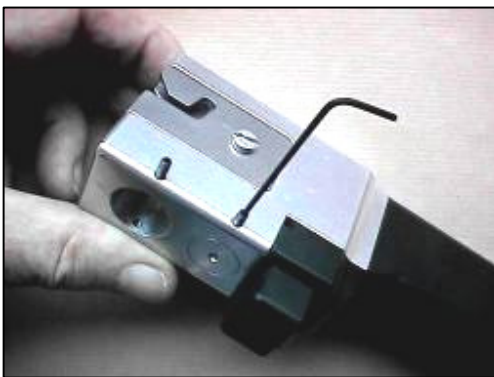
Figure 29. Removal of lower sealing plug
