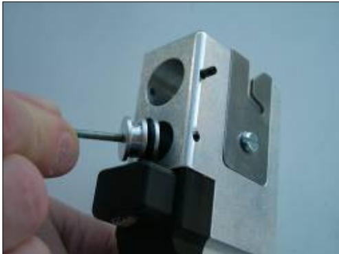
Figure 31. Knife piston plug removal
