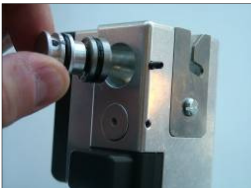
Figure 17. Top plug removal
