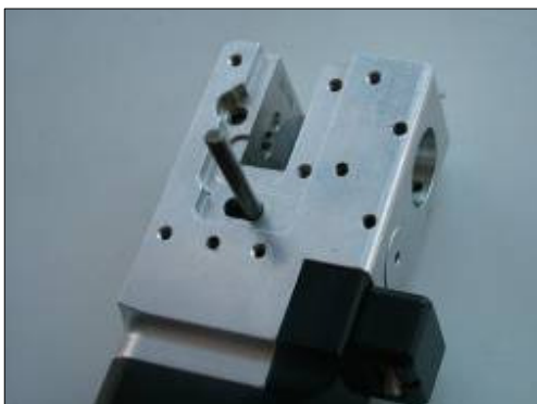
Figure 26. Knife assembly and extension block removed
