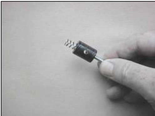
Figure 35. Knife drive piston assembly
