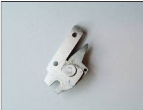
Figure 28. Knife assembly – pivot pin
