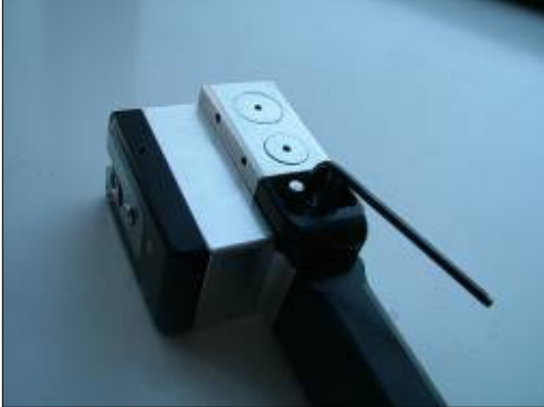
Figure 38. Release trigger housing
