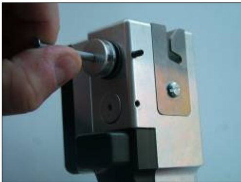
Figure 16. Top plug removal
