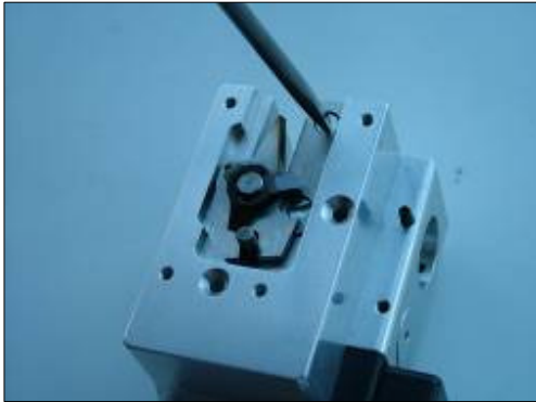
Figure 24. Knife assembly removal
