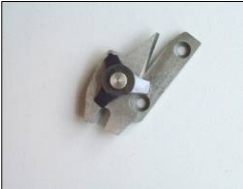
Figure 27. Knife assembly – detail
