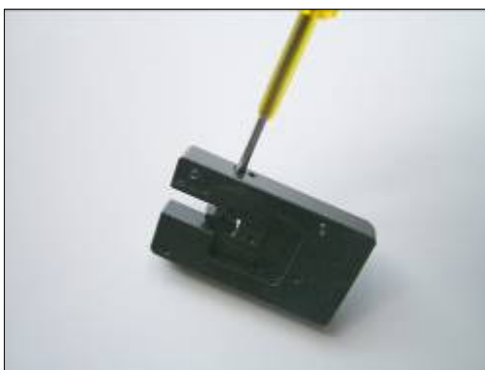
Figure 48. Release yarn clamp adjusting screw
