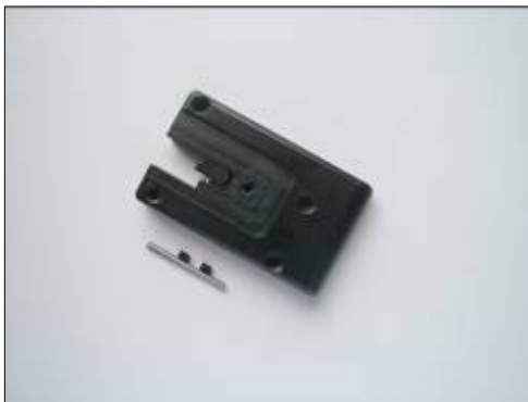
Figure 47. Remove yarn clamp stabilising pin
