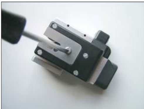
Figure 41. Remove yarn guide plate exit side
