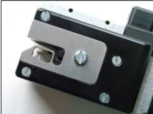
Figure 21. The more complex splicer side-cheek – fitted with yarn clamp
