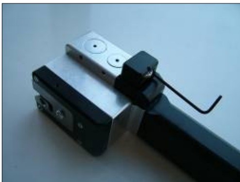
Figure 36. Removal of trigger button
