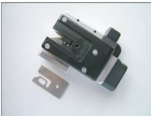
Figure 42. Yarn guide plate removed
