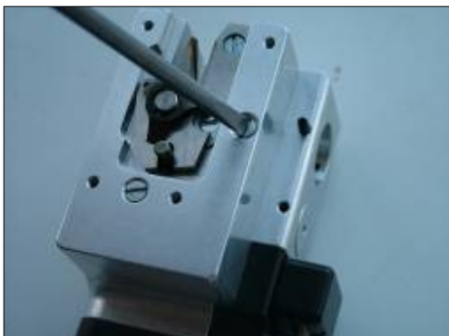
Figure 23. Extension block removal (part 1)
