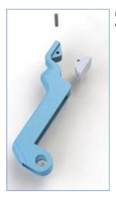
If required, press out the pad retaining pin, and separate the trigger and closure pad.
