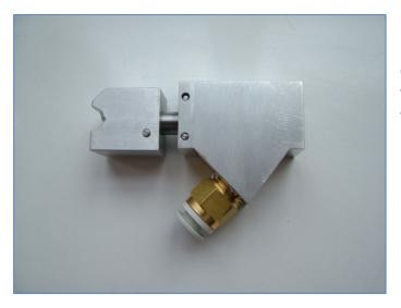
Lift the splicing unit out of the case, and detach the air feed tube, by compressing the quick-fit connector, and withdrawing the tube.
