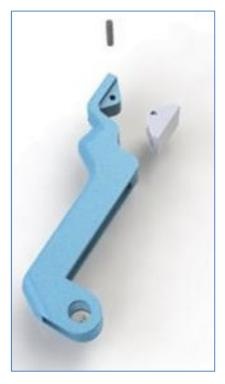
The closure pad mounting pin is an interference fit in the splicer trigger lever. This arrangement retains the closure pad, while allowing the pad to be a loose fit, so that it can align itself to the face of the splicing chamber.
