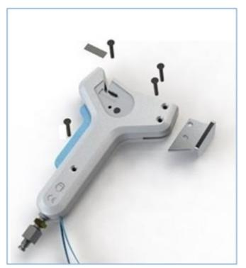
Place the splicer with its left side facing upward, allowing access to the three main slotted countersunk screws. Remove all three; removal of the top two allows the hanger (or the hanger blanking plate) to be removed.
