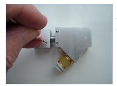
Remove the splicing chamber. With a small tool, press the chamber securing pin until it slides out. The chamber can then be removed from the valve.
