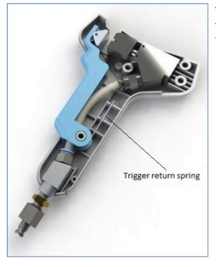
This action reveals the trigger return spring. TAKE CARE at this point; the trigger return spring may suddenly escape from its restraint location; sore fingers may result.
