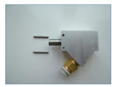
With the chamber removed, the compression washer can be seen; it is retained in place by two pins. Using the same small tool as before, press out the pins, so that they come free from the main splicer body.
