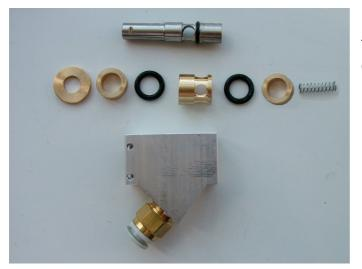
This photograph shows the splicer unit completely dismantled.
