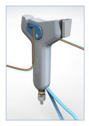
Hold the splicer in the left handBring yarns up beside the splicer, on the left hand side.Place yarns together into splicer; restrain with fingersAlternatively, restrain by looping round the index finger as shown below.
