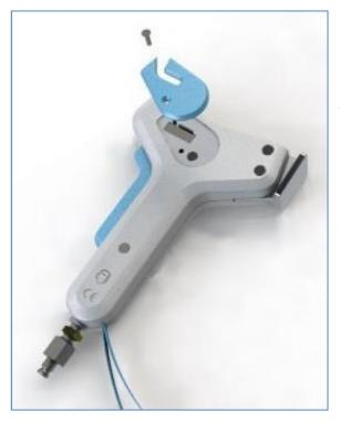
Once the side-plate is removed, the knife, Item 909, is exposed. It is held in a recess in the body. It can simply be lifted out of the body recess.
