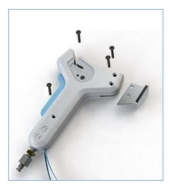
Return the splicer to its original position. This allows access to the four main slotted countersunk screws, M4 x 12 mm, Item 606, and M4 x 20 mm, Item 705.
