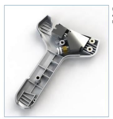
Place the splicer unit into the recess in the left outer case; ensure that it is seated snugly at the base of the recess.
