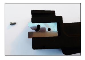
Removing yarn guide plate, yarn entry Side.
