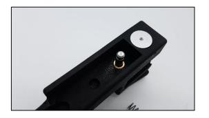
The main valve stem, Item 901 is now exposed, projecting from the splicer body.
