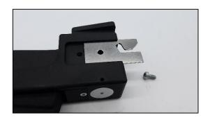
This shows the yarn guide plate, partly removed. Like the other plate, this one is restrained by a small moulding, and must be slid outward when being removed..
