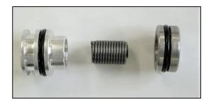
The pad is tethered to the upper sealing plug by an extension spring. The extension spring is screwed into the sealing plug, and the pad screwed to the spring. When the splicer has been dismantled, we recommend that the spring always be replaced.
