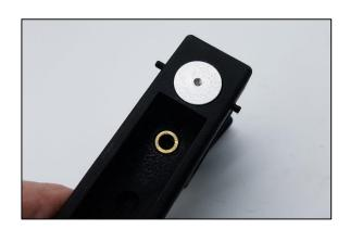
Removing sealing plug and chamber pad.
