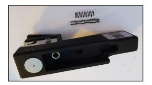
Splicer dismantling – valve assembly
