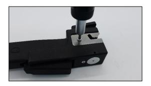
Removing the guide plate, exit side, Item 1031, and cutter blade, Item 909.
