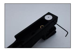
Removing sealing plug and chamber pad
