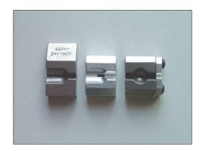
Bath-tubs are the chambers which are fitted most commonly to the Model 131/133/135.
