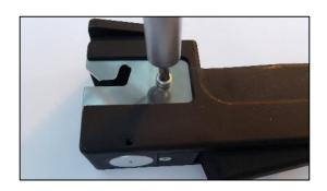
Removing yarn guide plate, yarn entry side.
