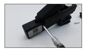
The trigger, Item 951, is secured by a pivot pin, Item 942, which terminates in a 2.5 mm hexagon socket.
