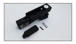
The trigger return spring Item 273, which fits into a circular recess in the splicer body, can now be lifted out.
