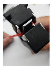
For a clean cut, the yarns must be pulled down sharply over the knife edge.
