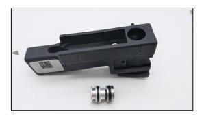
Removing sealing plug and chamber pad
