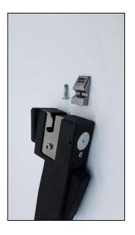
This photo shows the splicer with the splicing chamber removed.
