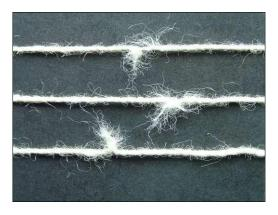
Ends-together splices, shown here., are suitable for lower-quality applications.
