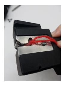
A completed splice emerging from the right-hand side of the splicer.
