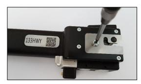
Removal of yarn guide plate, exit side.
