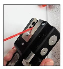
The splicer seen from the exit side. In some variants of the Model 133, the configuration on the exit side includes an adjustable yarn clamp; other variants have a plain exit plate, without a yarn clamp.
