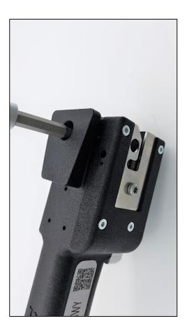
To release the splicing chamber, remove the single fixing screw Item 908 from the rear of the splicer body, when the splicing chamber can be lifted clear of the splicer.
