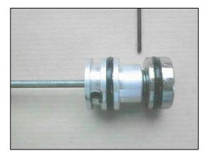
If the 'dry assembly' is satisfactory, dismantle and repeat the operation using adhesive. Apply a drop of Loctite Structural Adhesive 326 to the coils at one end of the spring, and screw the spring into the sealing plug until four or five coils of the spring remain exposed.
