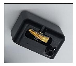
This photograph shows the trigger, detached from the splicer.
