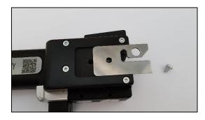
Removal of yarn guide plate, exit side.
