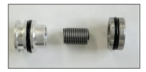
The pad is tethered to the upper sealing plug by an extension spring. The extension spring is screwed into the sealing plug, and the pad screwed to the spring. When the splicer has been dismantled, we recommend that the spring always be replaced.
