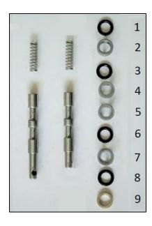
Removing valves, spacers, and O-rings
