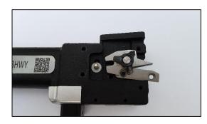
Removal of cutter sub-assembly.
