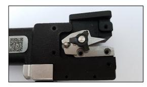
Removal of cutter sub-assembly.
