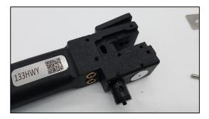
Removal of lower sealing plug and knife piston
