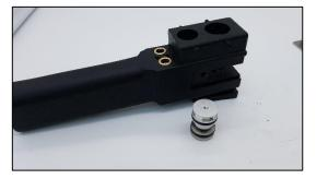
Removal of upper sealing plug and pad assembly
