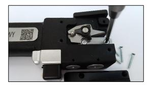
Removal of cutter sub-assembly.
