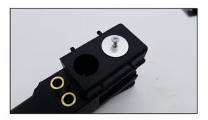
Removal of upper sealing plug and pad assembly
