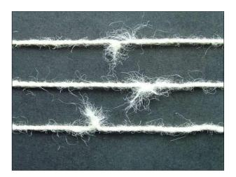
The 103 Series splicers make a joint of the "ends-together" form. This type of splice generally has a small tail but with excellent strength, whether used on "well-behaved" yarns such as multi-filament nylon, or on more difficult yarns such as those made from staple blends or highly twisted yarns.
