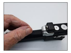
Removal of trigger button sub-assembly.
