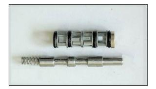
Removing valves, spacers, and O-rings
