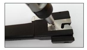
Removal of yarn guide plate, entry side.
