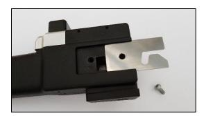
Removal of yarn guide plate, entry side.
