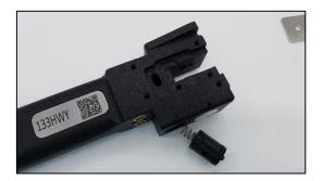
Removal of lower sealing plug and knife piston
