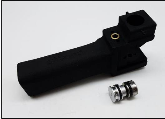
Removal of upper sealing plug and pad assembly.
