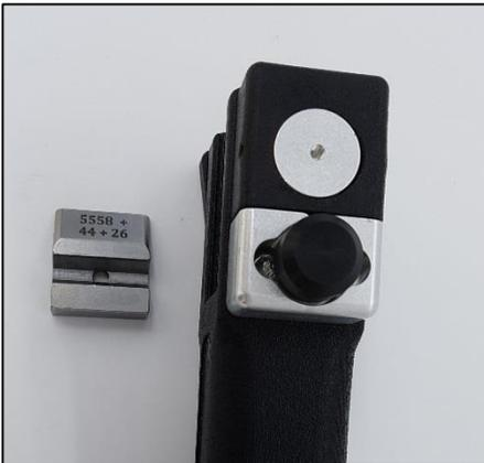
To release the splicing chamber, remove the single fixing screw from the rear of the splicer body, when the splicing chamber can be lifted clear of the splicer.
