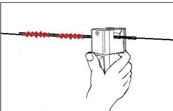
Repeat the splicing operation. Three splices over about 100 mm usually makes a satisfactory joint.
