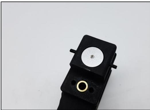
Removing upper sealing plug and pad assembly.
