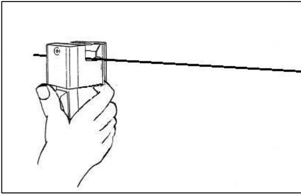
A Model 143 H splicer is shown here, as used by a right-handed operator. The splicer is held in the right hand, with the thumb on the trigger button.
