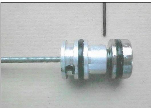
Apply more adhesive to the exposed coils of the spring and screw the pad onto the spring, ensuring that the gap between sealing plug and pad is roughly parallel and is between 1.5 and 2.0 mm. Allow the adhesive to cure for about 30 minutes.
