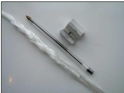
This photo shows the full potential of the Model 143; it is quite unique in that it is capable of splicing yarns up to around 9600 tex.
