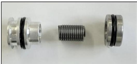
If the 'dry assembly' is satisfactory, dismantle and repeat the operation using adhesive. Apply a drop of Loctite Structural Adhesive 326 to the coils at one end of the spring, and screw the spring into the sealing plug until four or five coils of the spring remain exposed.
