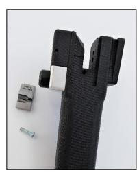
This photo shows the splicer with the splicing chamber removed.
