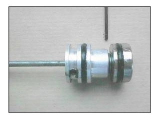
Check that the pad is approximately parallel to the sealing plug and that a gap of 1.5 to 2.0 millimetres between sealing plug and pad can be achieved. If the components are markedly out of parallel, discard the spring.
