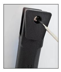
To release the splicing chamber, remove the single fixing screw Item 908 from the rear of the splicer body, when the splicing chamber can be lifted clear of the splicer.
