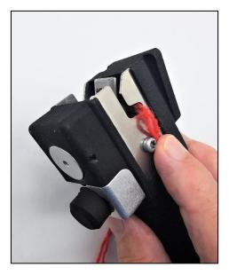
The yarns pass over the edge of the Knife on the left-hand side.
