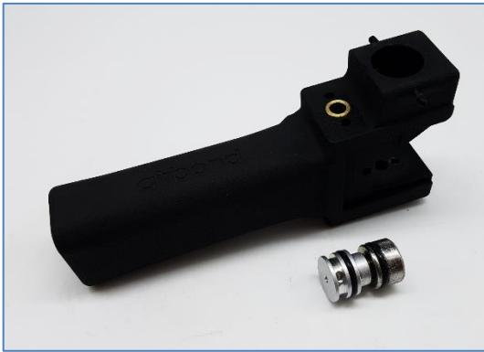
Removing sealing plug and chamber pad
