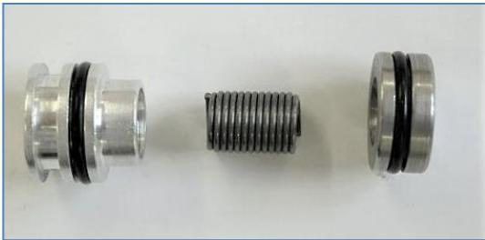
If the 'dry assembly' is satisfactory, dismantle and repeat the operation Using adhesive. Apply a drop of Loctite Structural Adhesive 326 to the coils at one end of the spring, and screw the spring into the sealing plug until four or five coils of the spring remain exposed.
