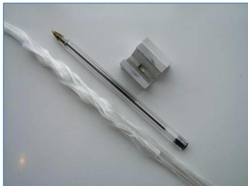
This photo shows the full potential of the Model 144; it is quite unique in that is capable of splicing yarns up to around 16000 tex.
