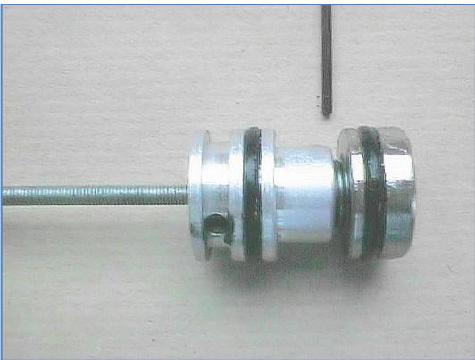
Apply more adhesive to the exposed coils of the spring and screw the pad onto the spring, ensuring that the gap between sealing plug and pad is roughly parallel and is between 1.5 and 2.0 mm. Allow the adhesive to cure for about 30 minutes.
