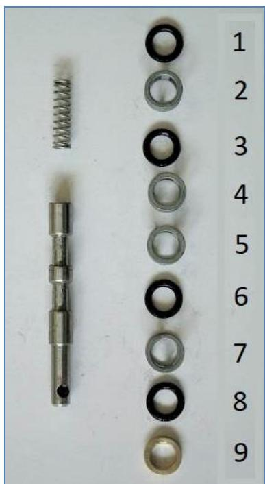
Sequence for reassembly; 1 – 9. First item placed in the bore is the O-ring, 1, Item 264, followed by the shell, 2, Item 276, and so on to the spacer, 9.
