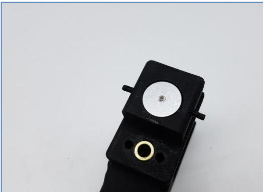
Removing sealing plug and chamber pad.
