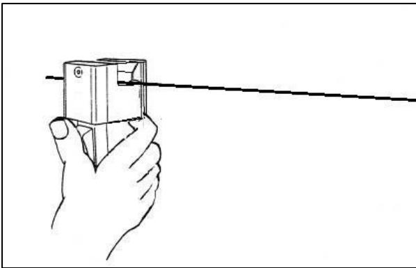
A Model 144 H splicer is shown here, as used by a right-handed operator. The splicer is held in the right hand, with the thumb on the trigger button.
