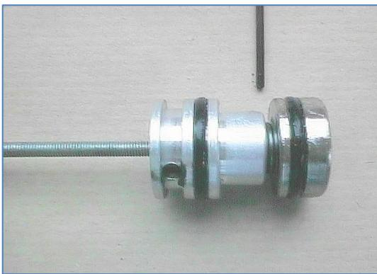
This photo shows the threaded rod method of extraction; the threaded rod can be seen at the left hand side.
