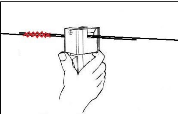
Press the trigger lightly, so that the pad closes, but no air blast emerges from the chamber. Check that the position of the yarn in the chamber is correct, and that the yarn can move freely through the chamber. Then press the trigger fully, so that the air blast starts. Move the splicer to the right, leaving the first splice exposed.
