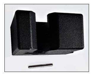
The knife drive shaft, shown after removal from the knife drive block.
