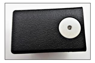
The sealing plug, Item XXX, has an M3 tapped hole. This is used to remove the plug once its securing screw has been removed.
