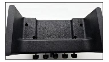
The underside of the splicer. This is notable for its simplicity; it is devoid of all tubes and fittings – features which were very evident on the earlier Model 122.
