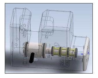
The knife drive block and SEALING PLATE, after the removal of the return spring.
