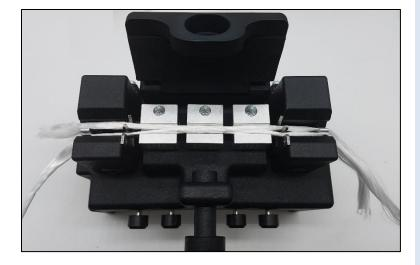
Select the first yarn. Take a length of yarn which is sufficient to pass through the splicer, leaving an excess length of about 5 - 10 cm.
