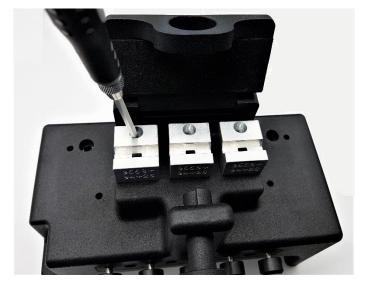
Removal of splicing chambers.
