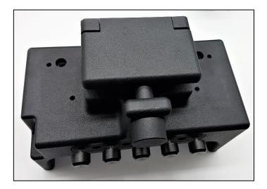
The splicer, after the knife drive blocks have been removed.
