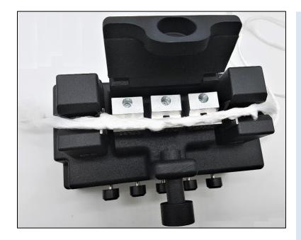
Close the lid, secure the cam and then press the 5 button sequence from left to right.
