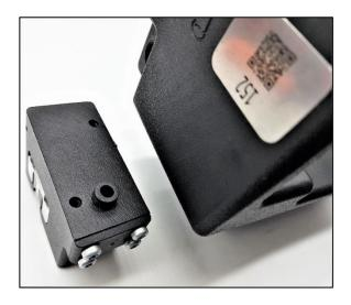
The knife drive block, after removal from the splicer chassis.
