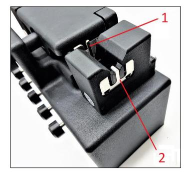
Each cutter motor block is fitted with two important sub-assemblies: The yarn cutters (here just visible, at position 1) The yarn clamps (at 2) These clamps
