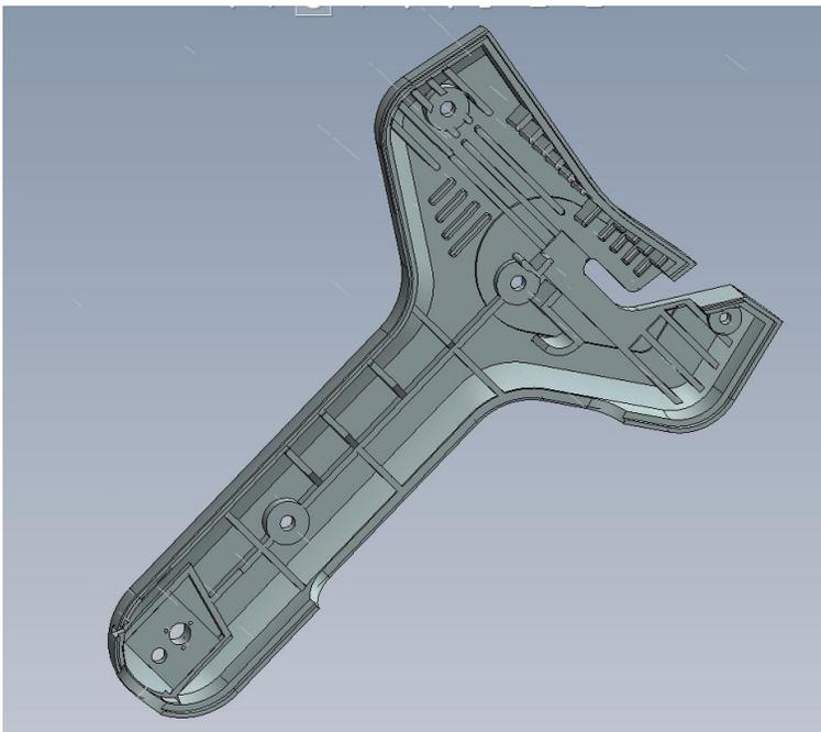
The inner surface of the lower shell of the 701 HF Series 2 splicer.
