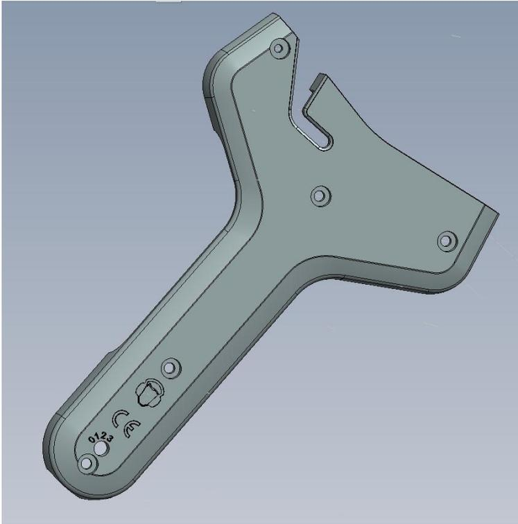
The outer surface of the upper shell of the 701 HF Series 2 splicer.
