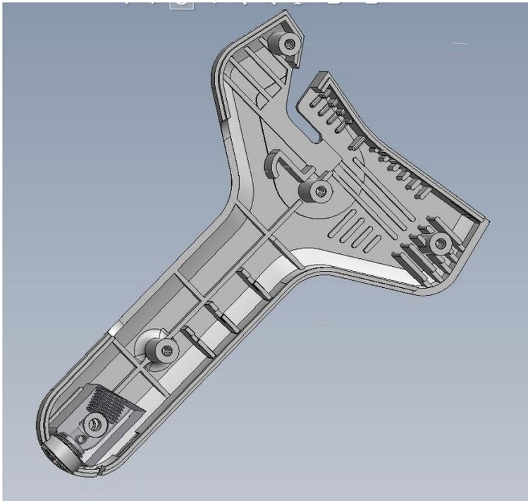
The inner surface of the lower shell of the 701 HFW Series 2 splicer.
