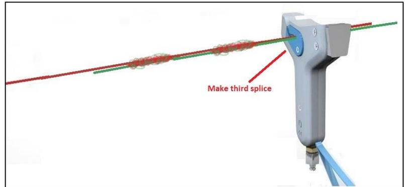
After the third splice, cut off the waste ends of yarn using a scissors.
