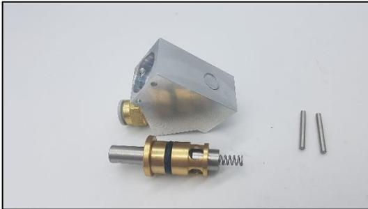
The inner assembly withdrawn from the splicer body.
