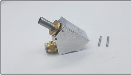
Grip the end of the valve, and gently withdraw the inner assembly
