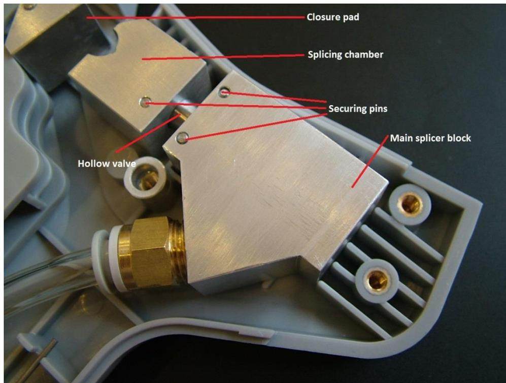
The closure pad is at the top left. The splicing chamber is secured to a valve which runs inside the main splicer block. The valve is hollow, such that air passing through the valve is directed into the chamber. When the chamber is in the resting position, the valve is closed, so that no air flows into the chamber.
