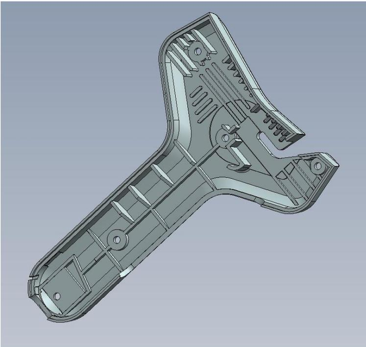
The inner surface of the upper shell of the 701 H Series 2 splicer.
