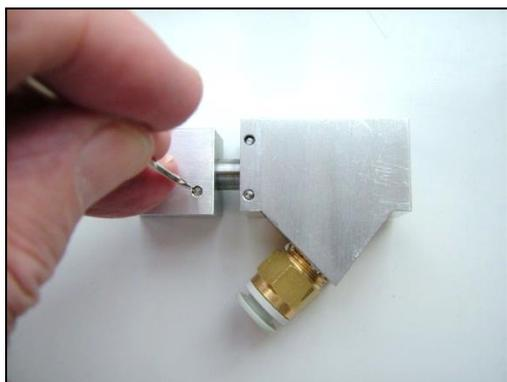
Remove the splicing chamber. With a small tool, press the chamber securing pin, Item 1604, until it slides out. The chamber can then be removed from the Valve, Item 1606.
