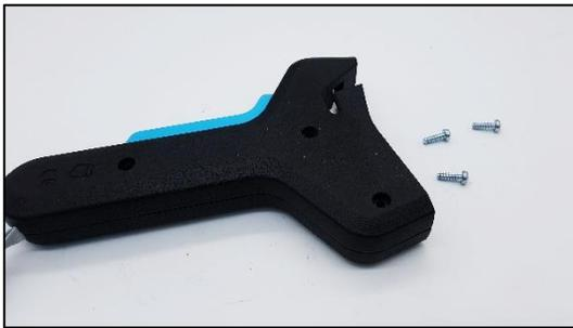
The splicer with three of the screws removed.
