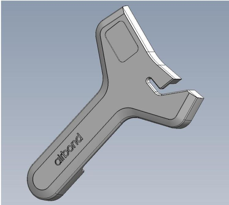
The outer surface of the lower shell of the 701 HF Series 2 splicer.
