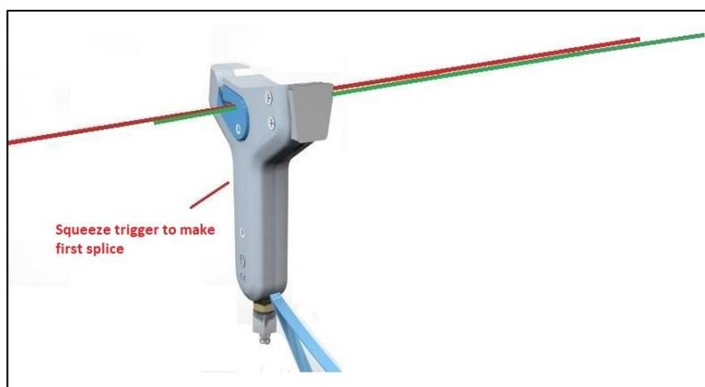
Once the first splice is complete, slide the splicer sideways by about 40 – 50 mm and repeat
