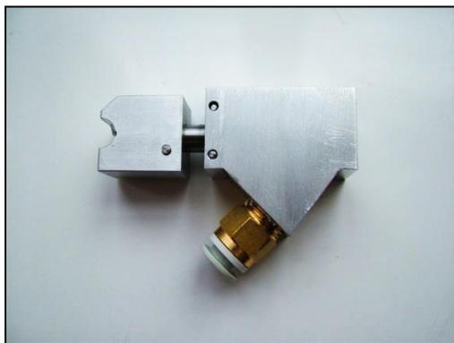
Lift the splicing unit out of the case, and detach the air feed tube, by compressing the quick-fit connector, and withdrawing the tube.
