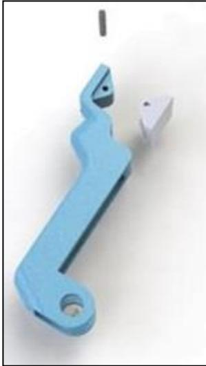
If required, press out the pad retaining pin, Item 1605, and separate the trigger Item 1614 and closure pad Item 1610
