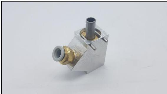
Using the same small tool as before, press out the pins, so that they come free from the main splicer body.
