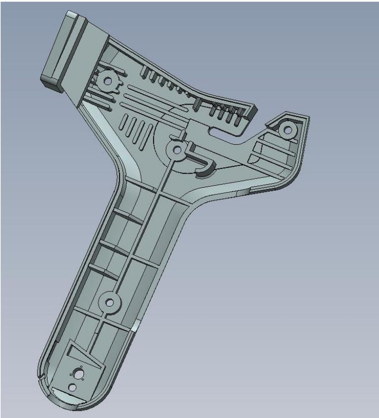
The inner surface of the upper shell of the 701 HFW Series 2 splicer.
