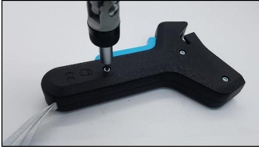
The body shells of the 701 Series 2 are held together by self-tapping screws, 4 x Items 1191 and 1 x Item 1194.
