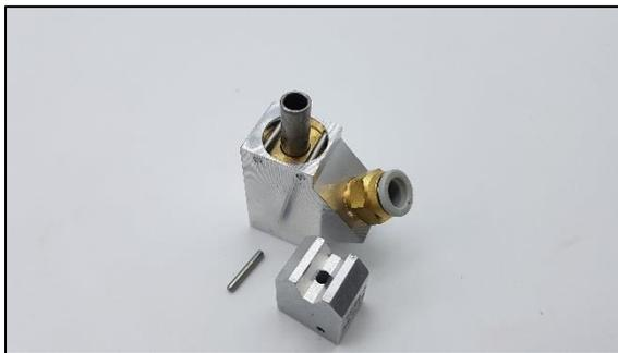
With the chamber removed, the compression washer can be seen; it is retained in place by two pins Item 1603.
