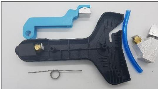
Here is the splicer with its principal components disassembled:
